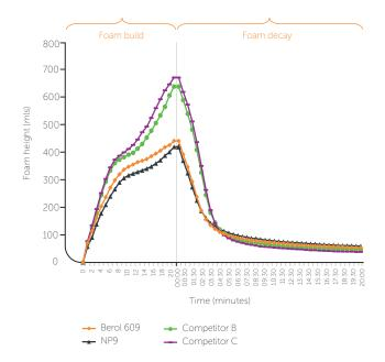
Berol 609 exhibits lower foaming than competitive NP9 replacers for better rinsability. SITA foam profile of 0.1% surfactant in water at 25°C (stirred 20 times @1000rpm for 10 seconds with foam height measurement each time, foam decay measured every 15 seconds over 20 minutes).
